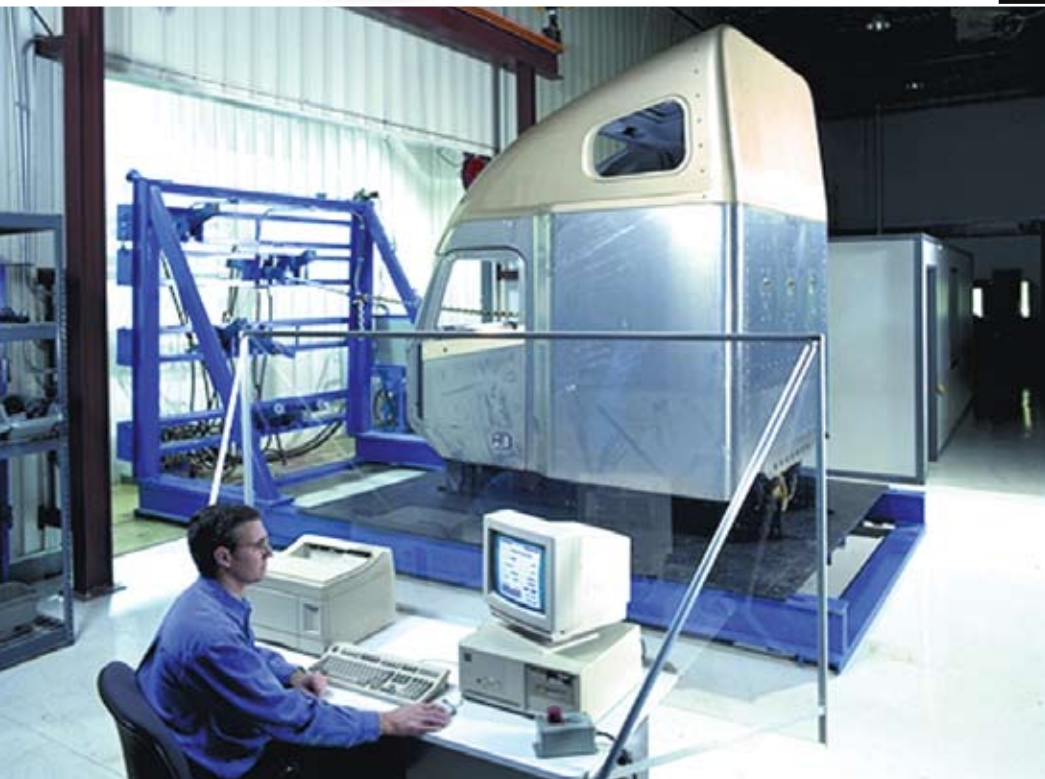
Full vehicle FMVSS 207/210 load testing
