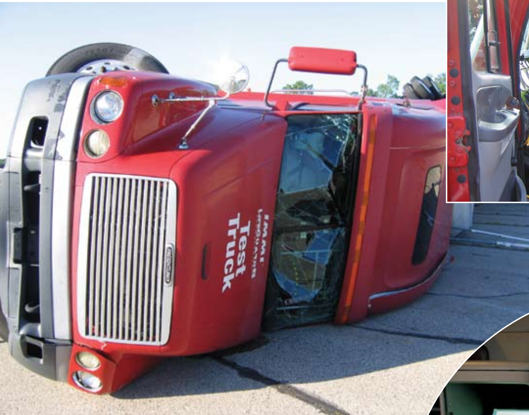
Remote control tractor-trailer rollover test
